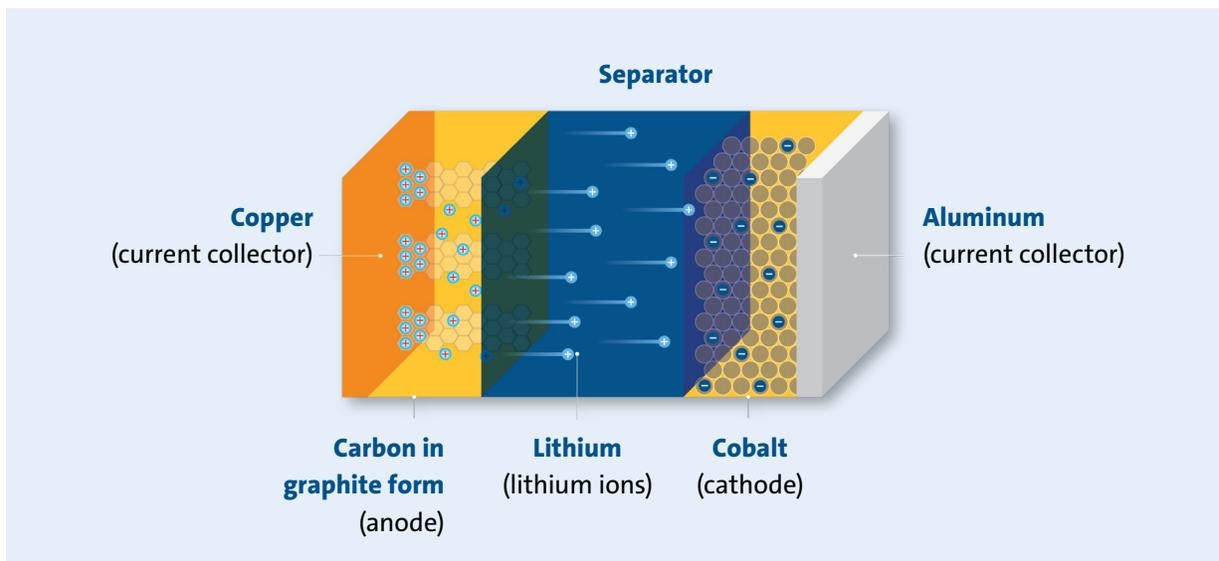
Li<sup>+</sup> ions move between the battery's cathode and anode internally, and electrons move in the opposite direction in the external circuit. This migration is the reason the battery powers the device, because it creates the electrical current.
